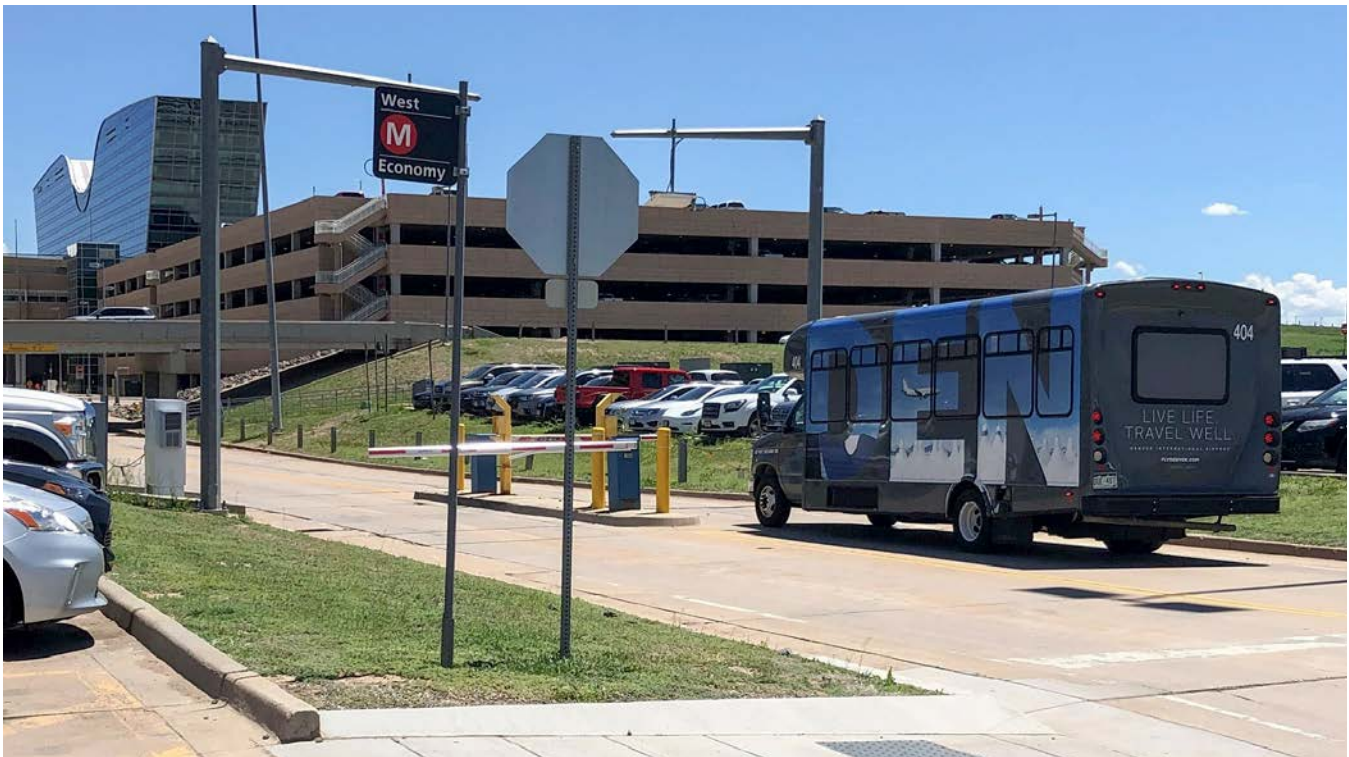
GATES FOR WEST ECONOMY LOT | An airport parking shuttle passes through the exit gate of the West Economy parking lot at Denver International Airport. The GateKeeper system records the time of all gate entries, which airport staff can then download to assess ABM Parking Services Inc.'s compliance with service-level requirements. PHOTO BY AUDITOR'S OFFICE STAFF
